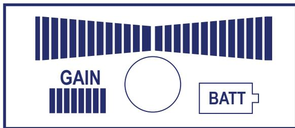
Signal Strength and Polarity (-) or (+) is indicated by the two opposite-facing bar graphs. The signal indications start in the center-most short bars and fill outwardly in increasingly larger bars as the signal increases, until maximum strength is reached.
